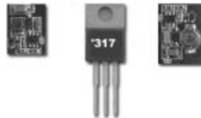
Figure 4. Tired of the Heat and Bulk of Linear Regulators? Switch! The Entire LT1616 Circuit Occupies Less Space Than a TO-220
